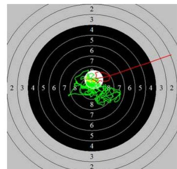
0.58 s of follow-through. The barrel moves directly to the right, compensates back a bit but there's definitely a balance/NPA Problem
